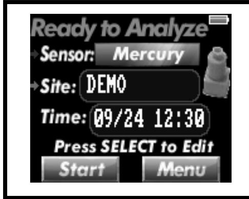
1. Press **ON/OFF** to initialize AND1100. Confirm correct Sensor and Site setting.
