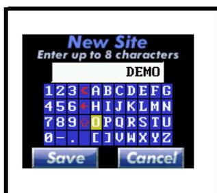
5. Press **ON/OFF** to initialize AND1100. Press **SELECT** and create a "New Site". (ex. "DEMO"). Unit will enter Site Calibration.
