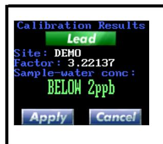
11. When prompted, remove cuvette to view and apply results. Discard all materials used.
